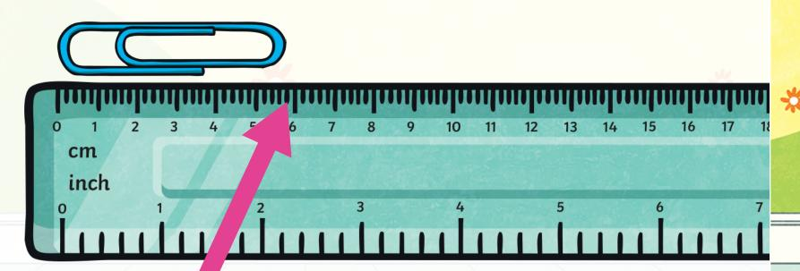
Count the number of intervals after the whole centimetre to find the length of the object to the nearest millimetre.
